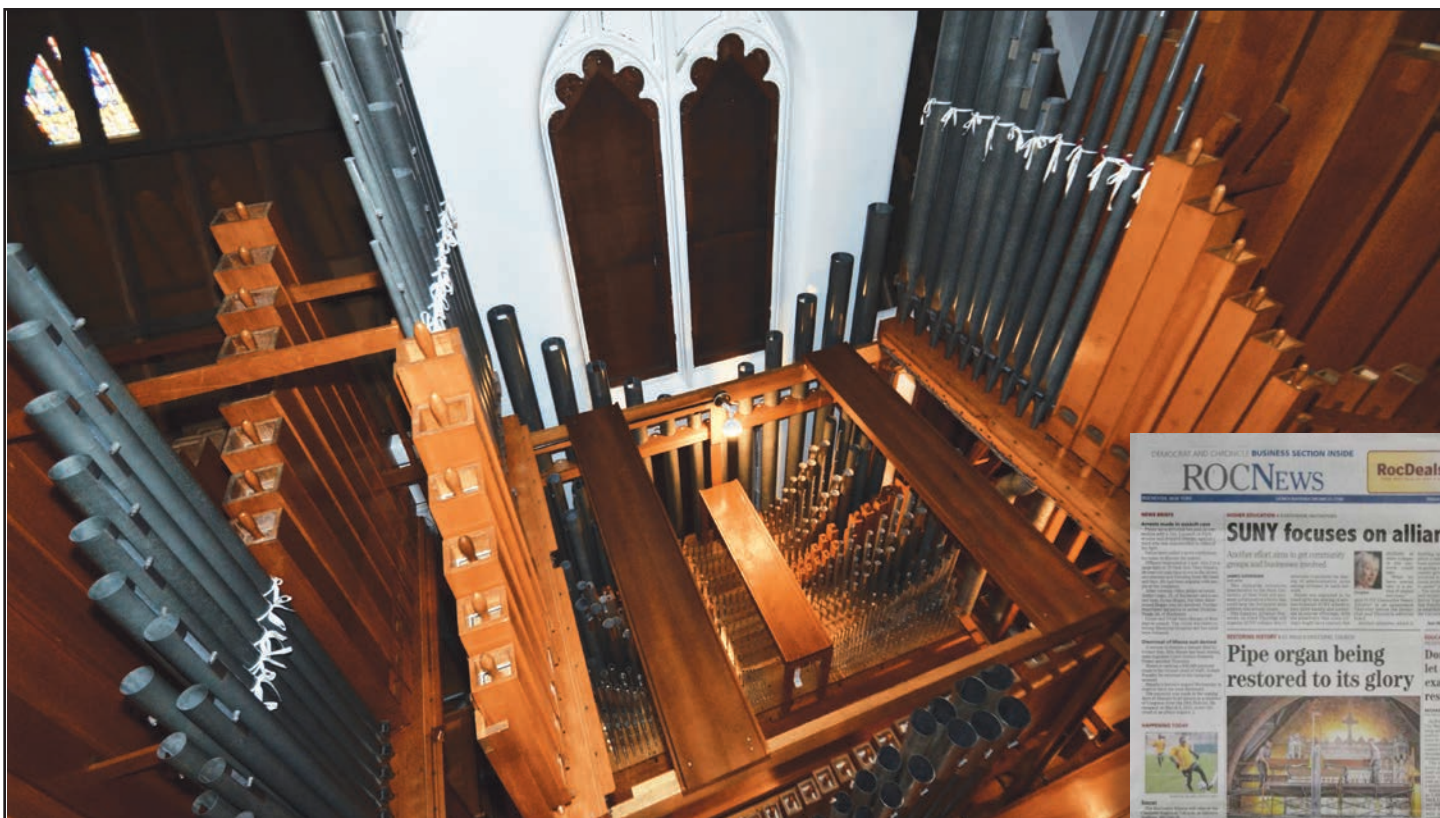
THE PEDAL & GREAT DIVISION PIPEWORK: This open division holds the two 32' ranks in St. Paul's two-story chamber, along with all unexpressive pipework (above). The Rochester Democrat and Chronicle reporting on the two year process of restoring this organ (right).
