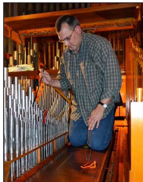
TONAL FINISHING: Duane Prill final tuning of the Great division Mixture pipes.
