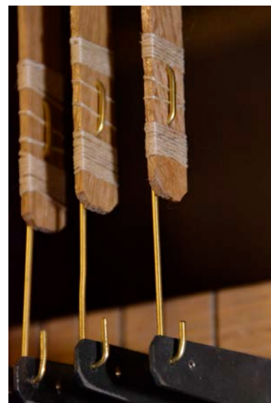
Detail view of tracker ends with hand-bent brass wires hooked into the squares
