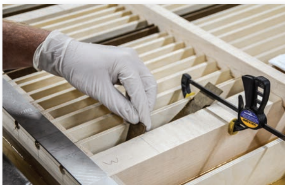
Installing dividers in tone channels for isolation of reeds and mixtures on slider windchests
