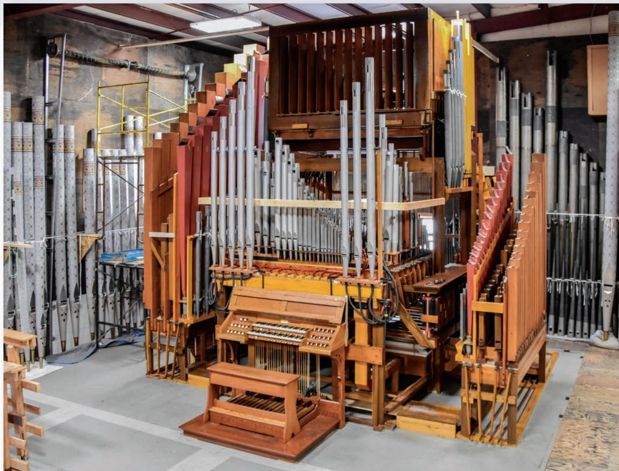
The organ set up in the workshop for testing without its case
